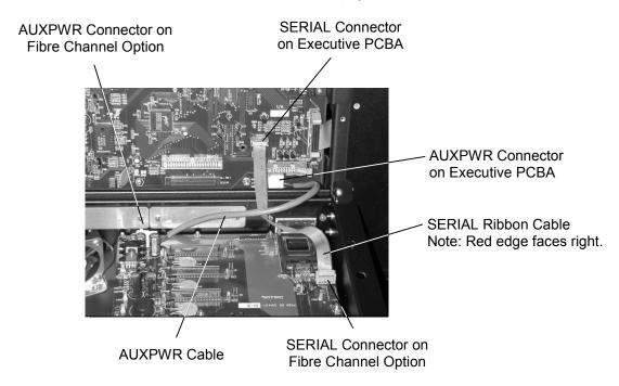
Figure 4-9 Detail of AUXPWR and SERIAL Connections (Executive III PCBA Shown)
